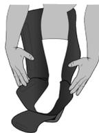
2. Open the leg and foot sections of the foam liner and place the foot and lower leg into the liner.
